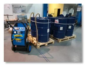
Oil filtration during service and filling with filtered oil
