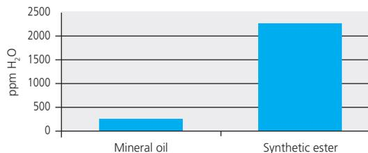
The water absorbing capacity varies from oil to oil. At saturation point (>100 % relative humidity), free water results in clouding.
