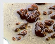
Damage by oil mixture leads to flocculation
