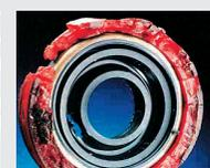
Bearing seal damaged by microdiesel effect
