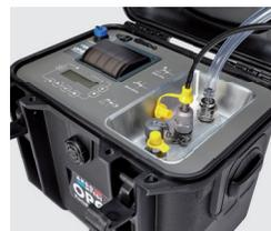
Automatic particle counters give a fast, accurate and repeatable contamination picture of your oil.
