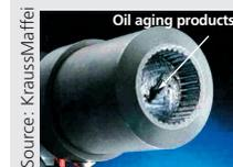
Clutch case damaged by oil aging
